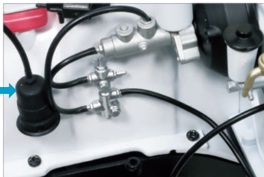
Insert the 24-H Rear Brake Pipe No.3 , fitted to the underside of the chassis in Issue 28, onto the right-hand protrusion of the 36-C Proportioning Valve .
