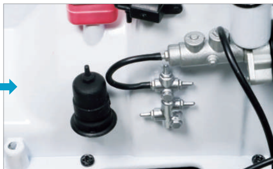
Insert the 37-I Front Brake Pipe No.1 cut in Step 1 onto the protrusion of the 35-I Brake Master Cylinder and the left-hand protrusion of the 36-D Front Brake Hose Connector .
