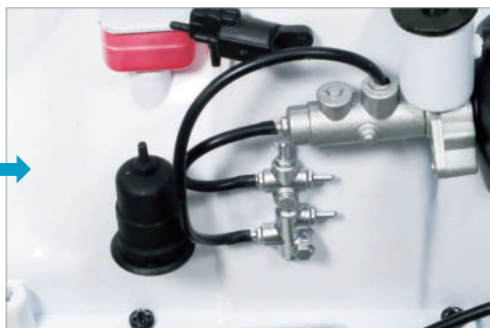
Insert the 35-M Rear Brake Pipe No.1 fitted in Issue 35 onto the left-hand protrusion of the 36-C Proportioning Valve .
